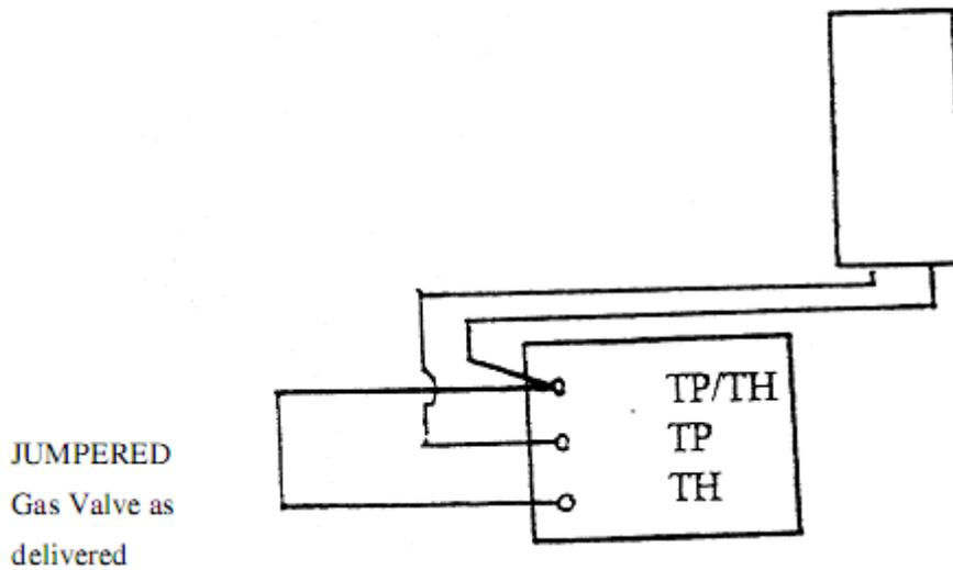
Remove factory jumper when installing remote control
