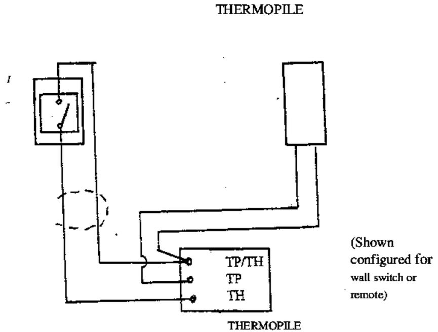
Note! Basket is delivered with Jumper wire installed. It must be removed for external switch or remote control to work.
